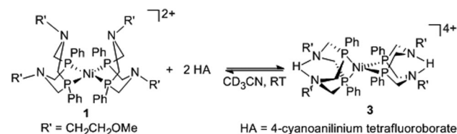
Scheme 2. Complex 1 is protonated in the exo position on each ligand upon addition of 4-cyanoanilinium tetrafluoroborate.
